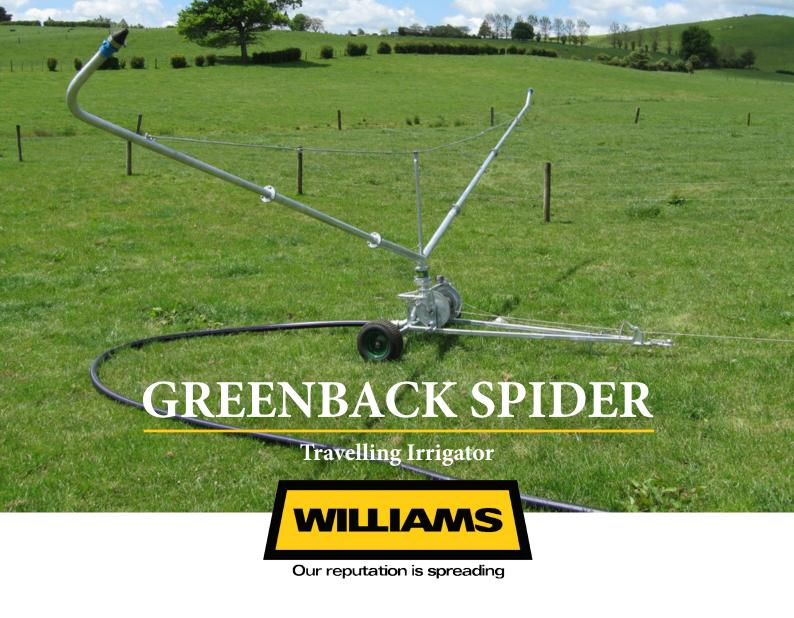
Increase your pasture production by capitalizing on your farms available resources with the Williams Greenback Spider Travelling Irrigator. A simple speed change procedure with a choice of five travel speeds, allows for greater control of effluent application depths (minimum of 5mm) thus optimizing the benefits of the natural fertilizer.
