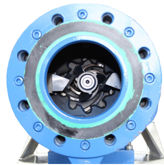
Double chopper system with a multi-channel impeller.
